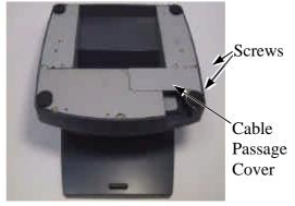
Now, remove the 2 screws on the cable passage cover and lift the cable passage cover away from the base, to show the passage.
